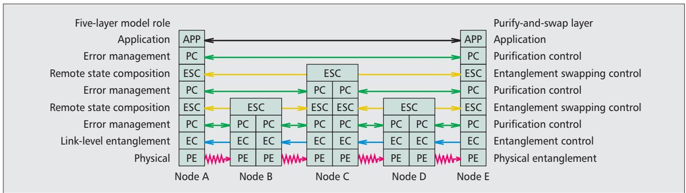
**Figure 4.** Protocol layers and their interaction in purify-and-swap repeaters in a five-node four-hop chain. The left labels indicate the model layer represented, and the boxed labels and right labels indicate the protocol name for purify-and-swap repeaters. Double-headed arrows indicate that bidirectional classical communication is required. Only the physical layer is quantum, shown propagating left to right.
